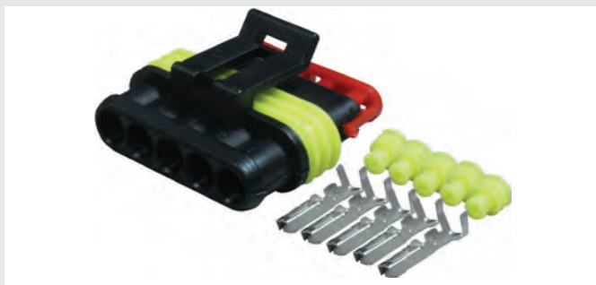
SSMF 5 Way Female SuperSeal Connectors Provides waterproof connection to IP67 Suitable for 0.5-1.5mm 2 Each pack contains enough terminals and seals
